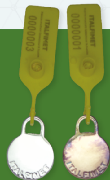
SAMPLES AFTER OXIDATION TEST: PASSIVATED SAMPE (LEFT) NOT PASSIVATED SAMPLE (RIGHT)
